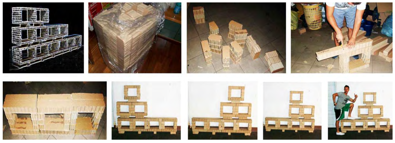
Fig. 7: Honeycomb cardboard bookcase prototype. Details of work in progress (Students: S. Esposito, F. Sorbino).
