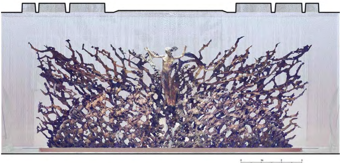
Fig. 2: La Resurrezione. Orthographic projection by point cloud model (Benecon).
