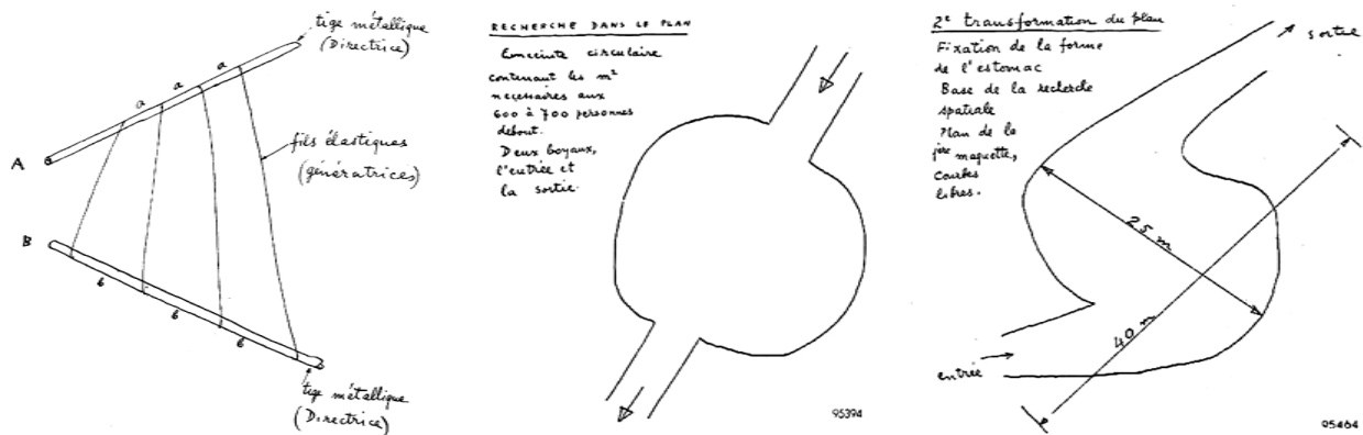
Fig. 3, 4, 5: Drawing of the tool used by Le Corbusier and Xenakis for the study of the hyperbolic paraboloids and first planimetric schemes by Xenakis.
