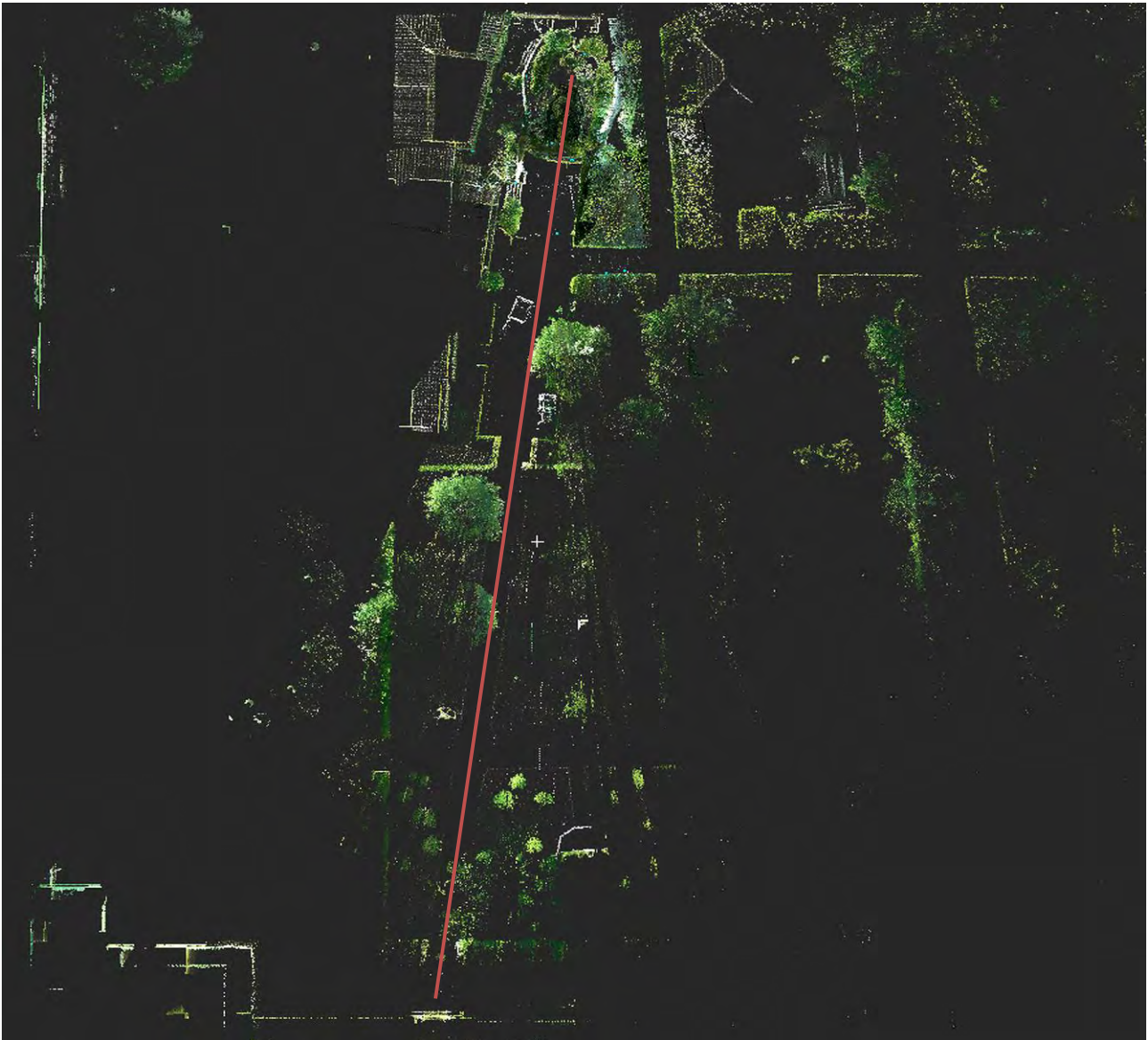
Fig. 2: Scanning laser collated; the elimination of tree species in the editing highlights the alignment of the fountain.
