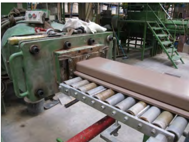
Fig. 1,2: Industrial processes of clay extrusion and cutting.
