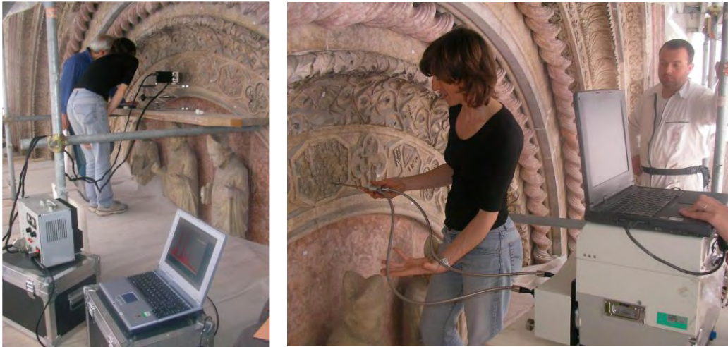
Fig. 1: experimental set-up for in situ measurements at the Palazzo dei Priori by XRF (a) and mid-FTIR (b)
