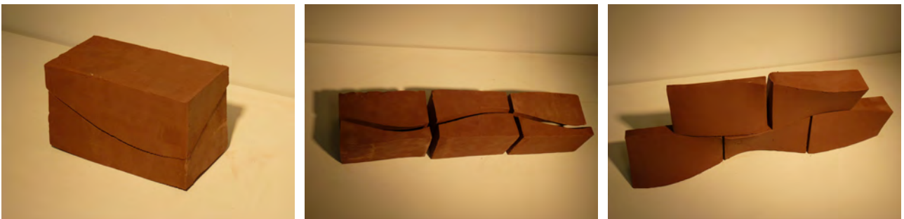
Fig. 7: Single components of unfired (green) terracotta and assembly simulation of a doubly-curved wall section.
