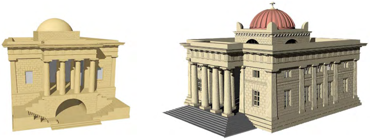
Fig. 5: Two perspective views of the digital models compared of Gymnasium . On the left, the first design hypothesis, that was never built; on the right, the current state.
