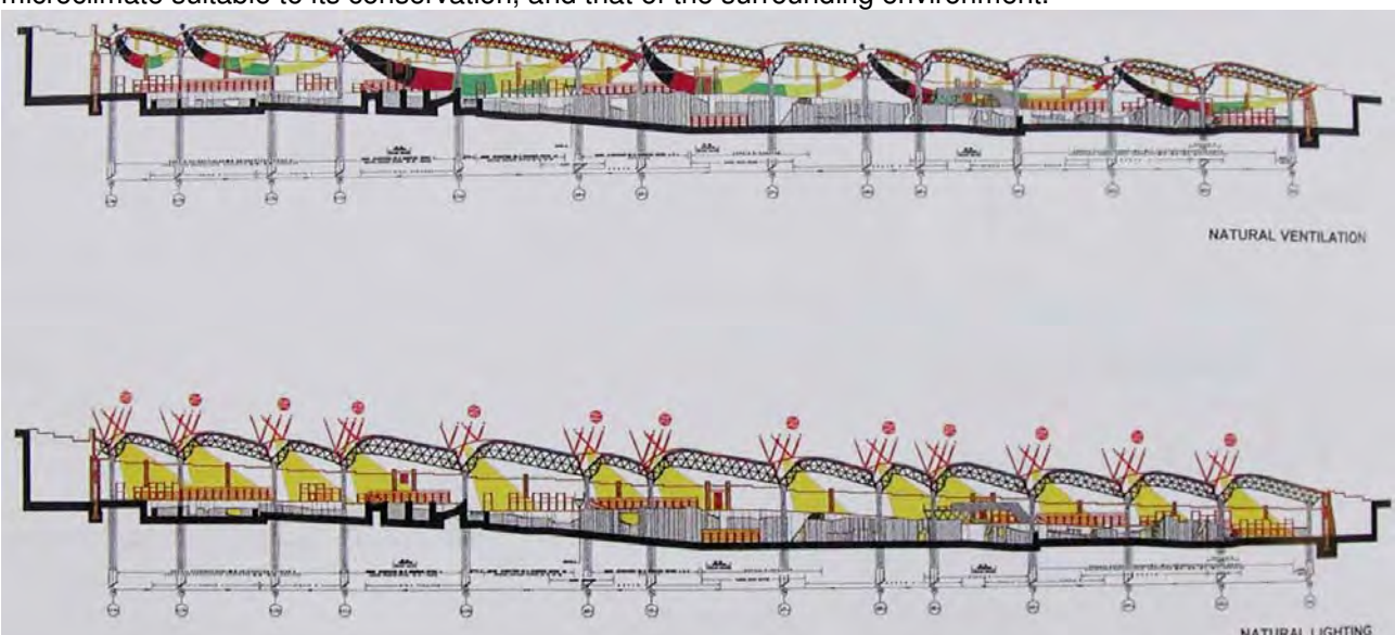
Fig. 17: Santorini, Akrotiri, sections through the protective structure, highlighting the systems of natural ventilation and illumination [De Matteis 2002, p. 92].
