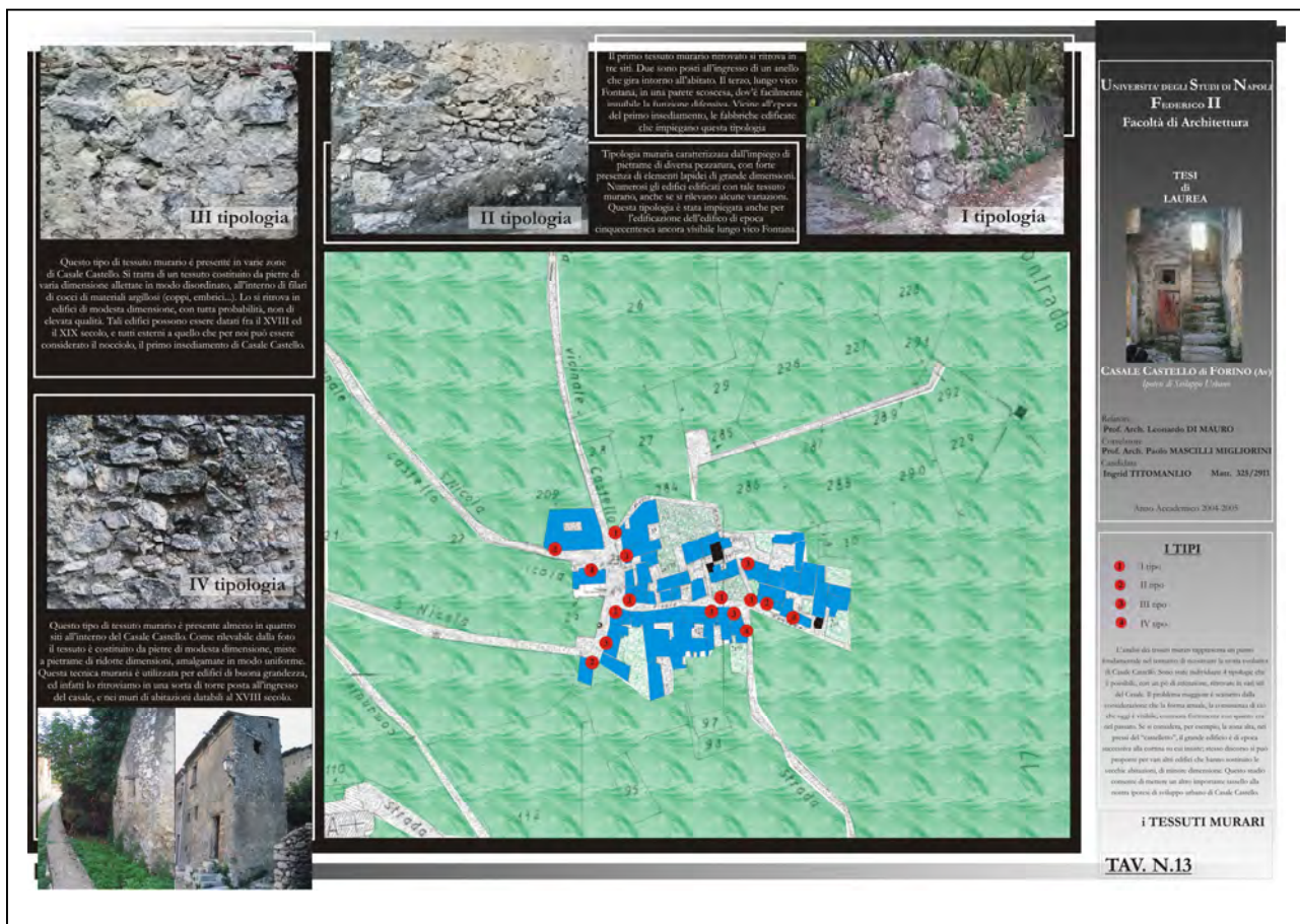
Fig. 1: Casale Castello: Analysis and classification of masonry coursing pattern
