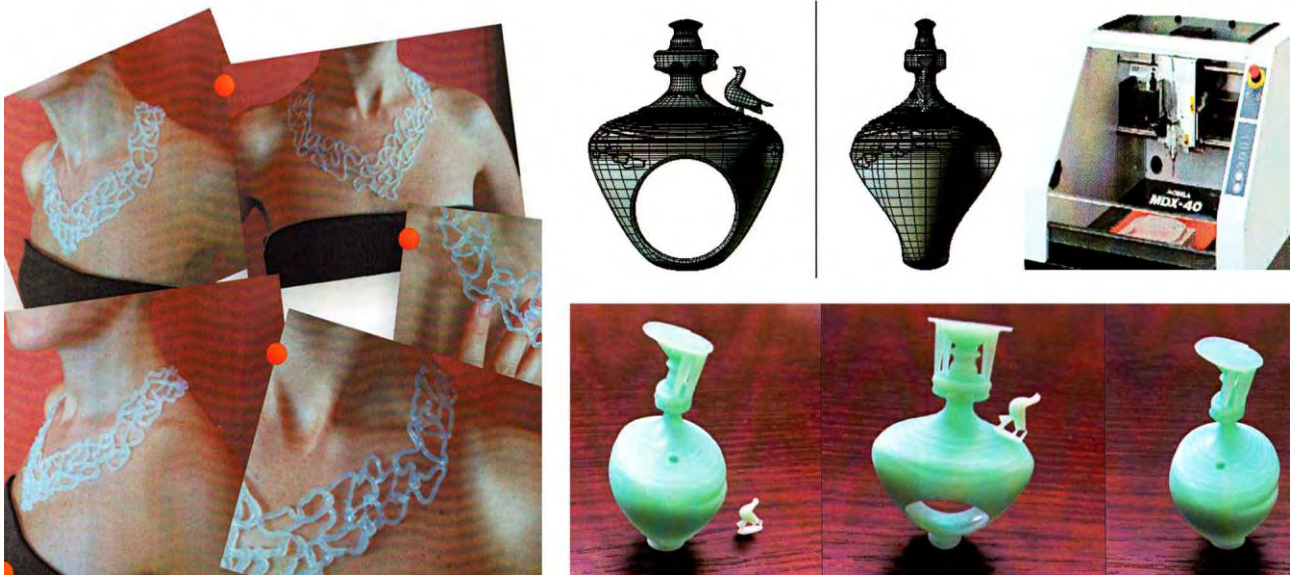
Fig. 9, 10: On the left, a collier realized by the straining of silicon rubbers in ad hoc made mould (Student: B. Frettoloso). On the right, renders and wax models of rings inspired to campanian etrusian archeology, realized by the laser stereolithography (Student: L. Gambero).
