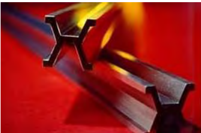
Fig. 8: International Prototype Meter standard bar, made of platinum-iridium, used as standard until 1960.
