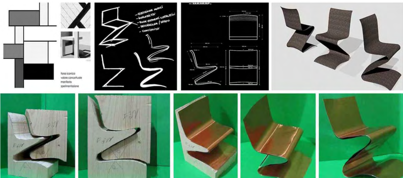
Fig. 2: The Tape Chair 2010 Design is conceived in carbon fibre, along the lines of the Zig - Zag revisitatio to which it adds the Panton Chair shapeliness, but the prototype, in reduced scale, has been realized in copper foil.
