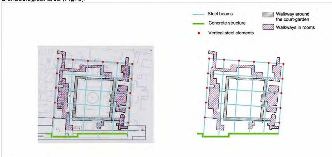
Fig. 3: Périgueux, domus de Vésone, diagrams of the structure and the paths inside the new protective structure.
