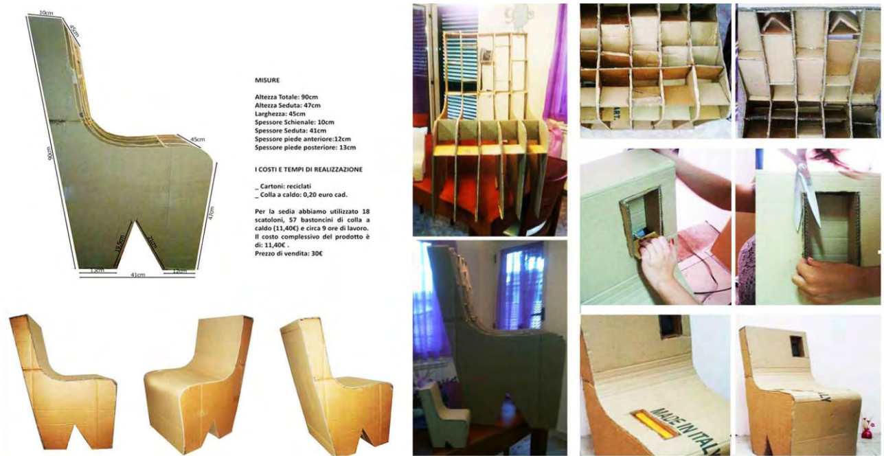
Fig. 6: Cardboard Comfortable Armchair Design. Specifications and prototype. On the right, details showing work in progress (Students: L. Palumbo, R. Chiarolanza).
