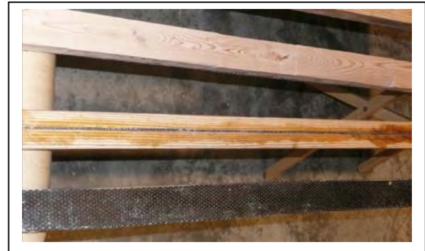
Fig. 14,15,16,17: Loose blocks epoxied to a 1.5in. carbon fibre tape in various arrangements from bent causing the blocks to spread and become quite flexible, to very rigid as the blocks come into contact and meet compressive forces. The stick spanning the chair and table will easily support a 200lb. person – the table is likely the weakest element. The three sticks at the right are: at the top a series of blocks with a tape below; the center stick has a 1.5in tape inserted into a saw cut; the bottom stick has the tape fully covering the face. With the tape on the side opposite the force, each will resist more strongly than a plain stick without the tape. Note: the loose blocks do not even need to be attached to the tape toward the center of the span – The tape requires a sound connection to the end blocks only. Attachment to several at the ends helps distribute the adhesive bond strength. A mechanical attachment to the end blocks would relieve the need for any adhesive.
