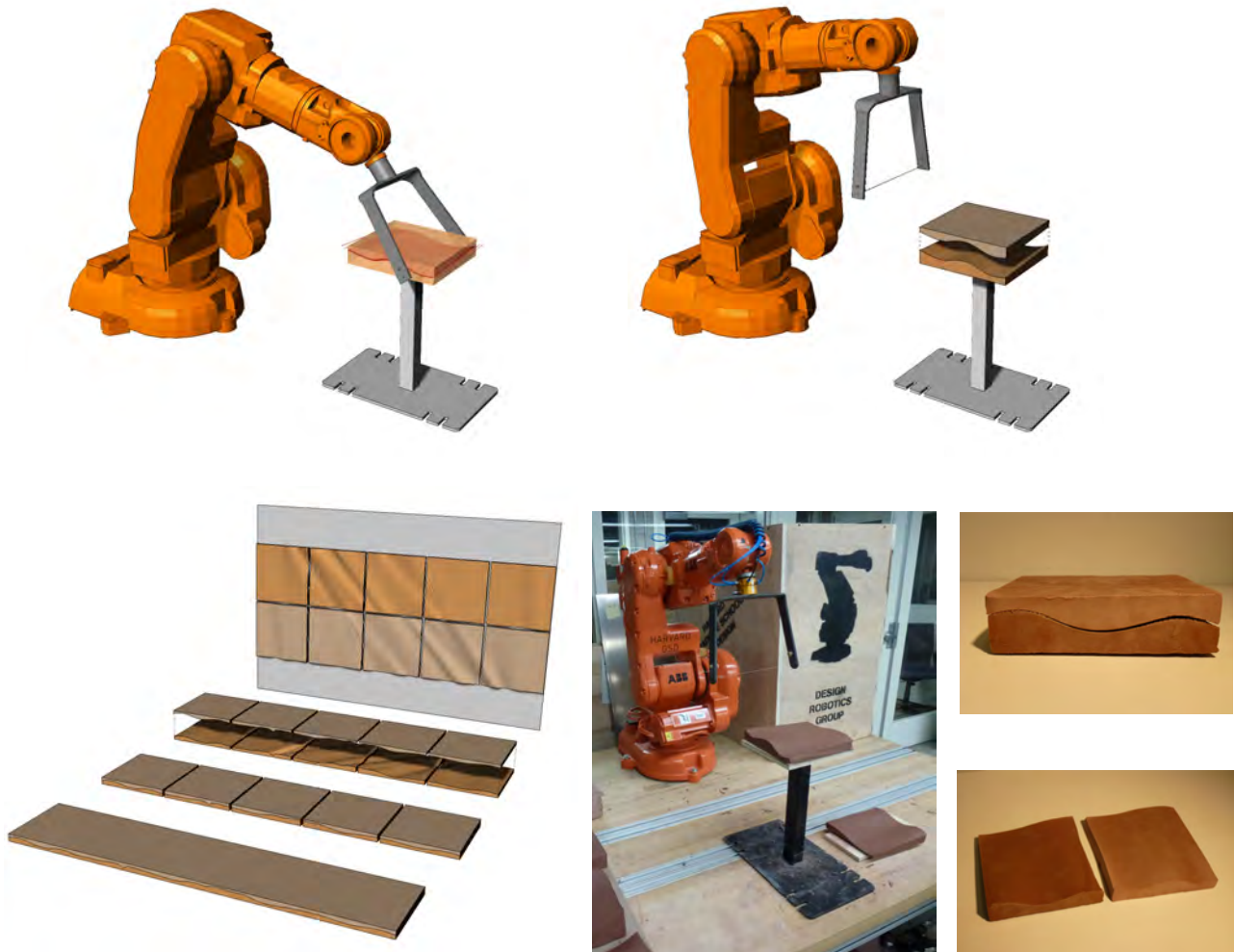
Fig. 9: Design speculations and robotic fabrication of complex terracotta tiles.
