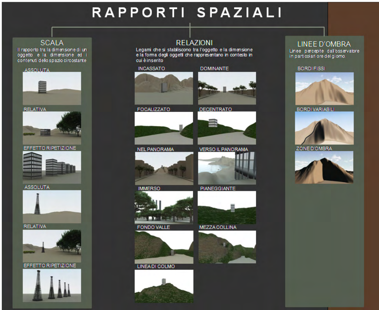
Fig. 9: An iconographic repertory of the most frequent and recognizable scale of relationship between built elements and landscape forms.
