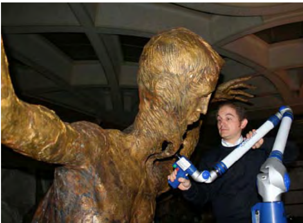
Fig. 35-36: 3D laser scanning action and mesh 3D model by point cloud model (P. Argenziano, Benecon 2011).
