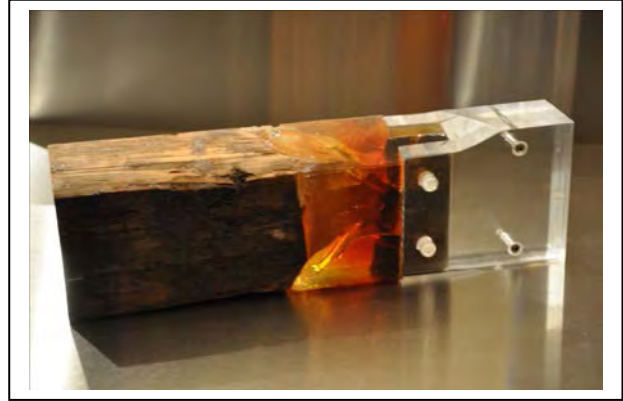
Fig. 18,19: Two views of the initial concept model for the glass prosthesis. The fragment of old wood is not from Menokin and salvaged from an urban trash container. It happened to have an angled top face and thus the top of the prosthesis was beveled at the point of contact. This would not likely occur in actual usage but obviously can be accommodated. The Prosthesis in the model is acrylic.
