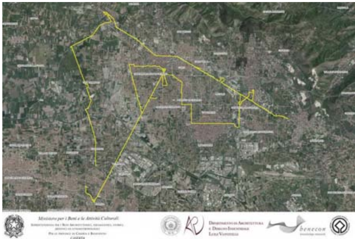
Fig. 5: Management Plan of the UNESCO site "Royal Palace of the eighteenth century in Caserta with the Park, the Aqueduct of Vanvitelli and the complex of S. Leucio. " Path surveyed by platform Topcon IP-S2 Mobile Mapping installed on a dedicated vehicle.
