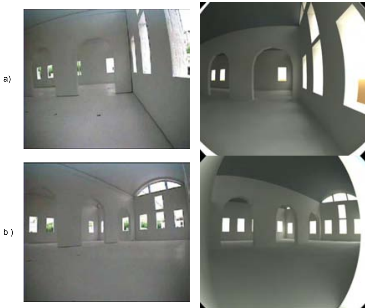
Fig. 8: Internal light distribution comparison scale model (left) vs. Radiance (right), for two building area, a) and b).
