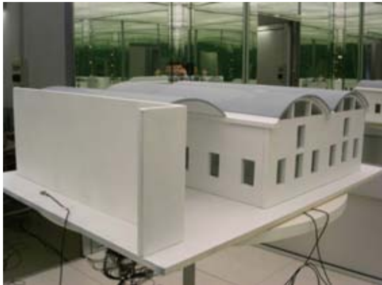
Fig. 3: Scale model of “Opificium” for acquisitions in the artificial sky.
