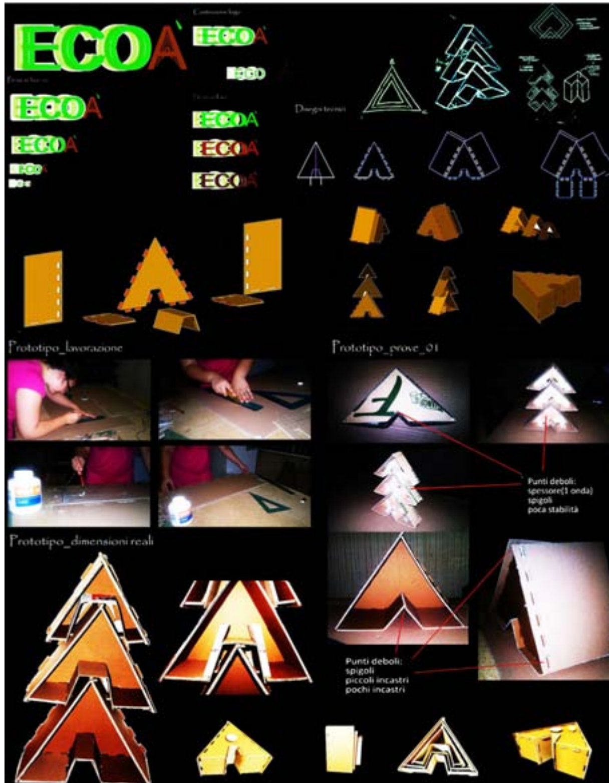
Fig. 6: Design of a recycled cardboard reversible book case - table: sketches, drawings, virtual renderings, prototypes. This project has been drawn and made by students of SUN | Second University of Naples_ Department of Architecture and Industrial Design_Course of Prototyping.
