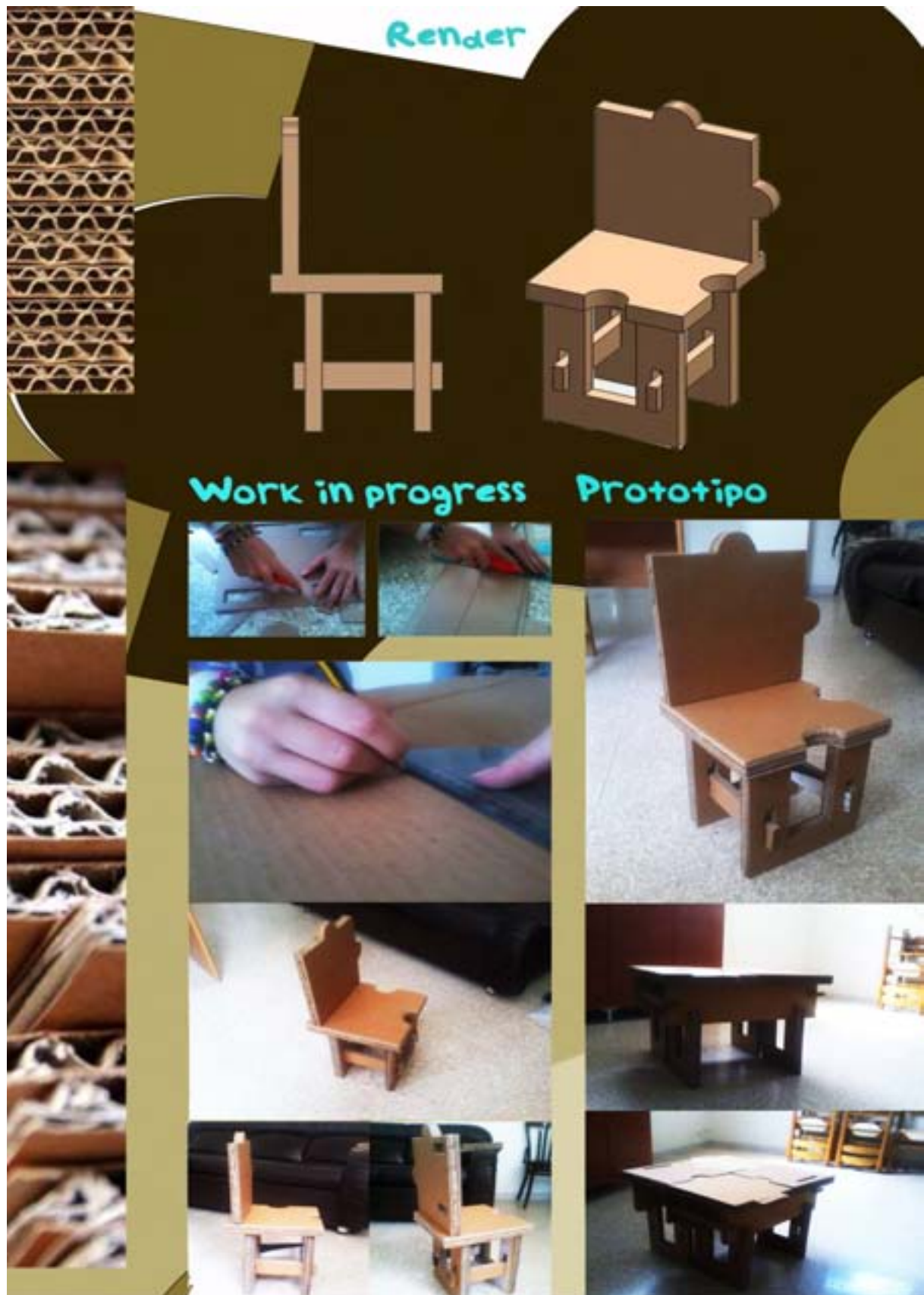
Fig. 14: Puzzle Pieces' Design. Work in progress of laboratory method and prototypes of recycled cardboard preschooler furniture based on the modular principle of puzzle's pieces made by some students of SUN | Second University of Naples_ Department of Architecture and Industrial Design_Course of Prototyping.
