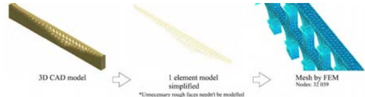
Figure 8: Modeling Process. From 3D CAD model to Mesh .med file in preparation for FE study.
