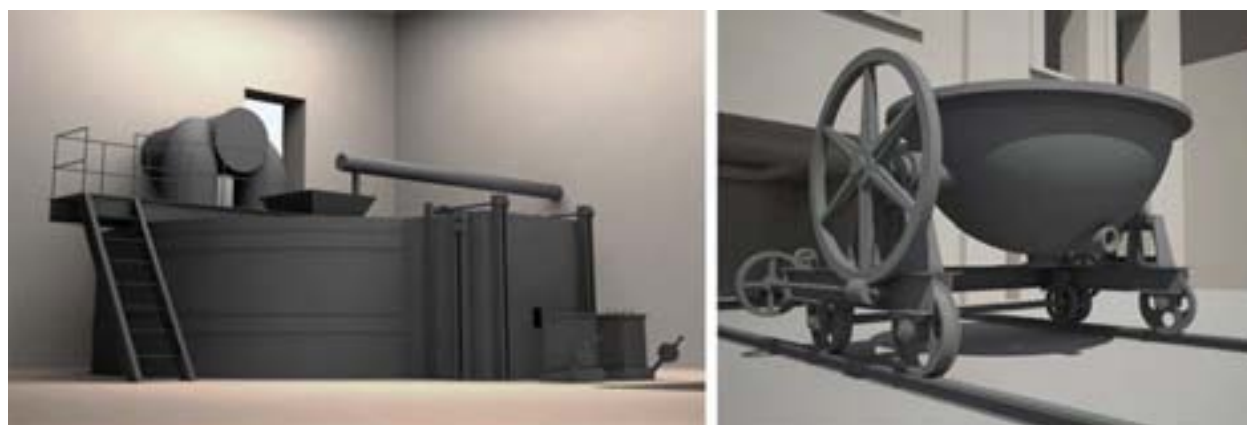
Fig. 10: The digitally reconstructed main furnace (left) and speiss converter (right).
