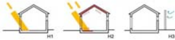
Fig. 10: Bioclimatic design strategies of the traditional courtyard house during heating period
